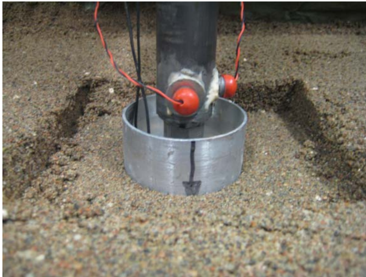
FIG. 2 – End of compaction with no observable heave.
